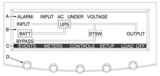
Figure 7-3. Parts of the LCD
